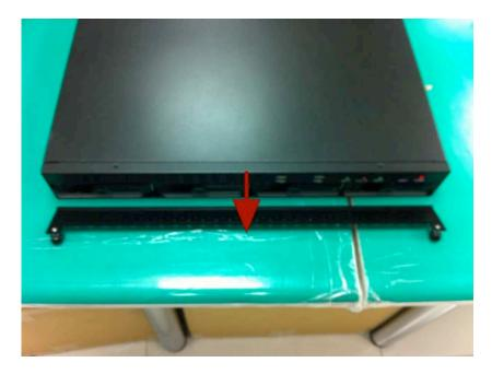
Simply pull to remove the front plate once the screws are loosened from the unit.
